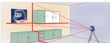
Ideal for alignment works, as tiles and cabinet installation
